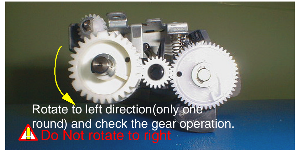
Figure 4-177. Checking Operation After Assembling "ASF Unit"
